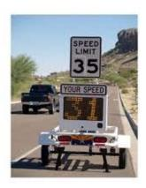
A device that consists of a changeable speed display, a radar speed detector and a regulatory speed limit sign. The speed control device encourages speed limit compliance.
