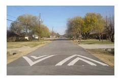
Speed humps are rounded raised areas placed across the road. They are generally 12 feet long (in the direction of travel), 3 to 3 ½ inches high, parabolic in shape, and have a crossing speed of 15-20 mph. speed humps on roadways with mike lanes should have a sinusoidal profile. When placed on a street with rolled curbs or no curbs, bollards are placed at the ends of the
